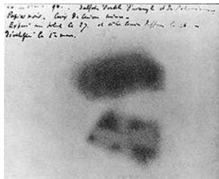
Image of Becquerel's photographic plate. The shadow of a metal Maltese Cross placed between the plate and the uranium salt is clearly visible.
